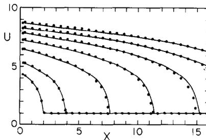
FIG. 2. Exact solution (—) versus numerical SSI solution (•) at equal time intervals;  $\varepsilon_1=0.1$ ,  $\varepsilon_2=0.08$ .
