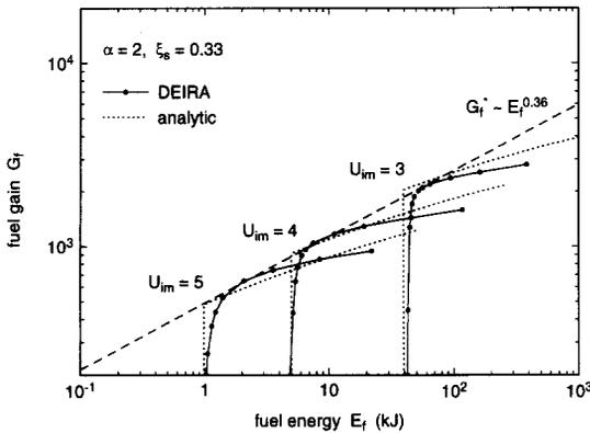
Fig. 3. Gain curves calculated for three implosion velocities with one-dimensional code DEIRA, by varying  $H_s$  for fixed  $T_s = 7$  keV and  $\xi_s = 0.33$ . Also shown are the analytic results (---) obtained with the aid of the ignition condition of Eq. (18), and the limiting fuel gain  $G_f^*$  (—).
