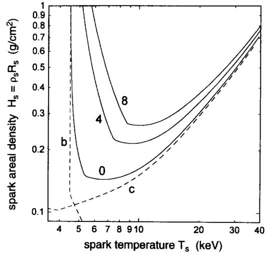
Fig. 2. The full curves show three ignition boundaries for spark parameters as defined by Eq. (17) for three different values (0, 4, and 8) of the right-hand side of this equation (in units of  $10^7 \text{ cm s}^{-1}$ ). To the right hand side of the dashed curve b, the alpha-particle heating  $Q_x$  exceeds the bremsstrahlung cooling  $Q_{br}$ . Above the dashed curve c, the alpha-particle heating  $Q_x$  exceeds the heat conduction cooling  $Q_{ec}$ .
