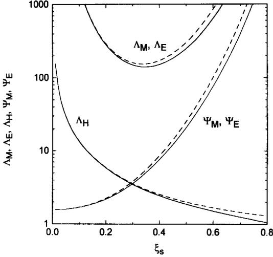
Fig. 1. Dimensionless functions  $\Lambda_M(\Omega, \xi_s)$ ,  $\Lambda_E(\Omega, \xi_s)$ ,  $\Lambda_H(\Omega, \xi_s)$ ,  $\Psi_M(\Omega, \xi_s)$  and  $\Psi_E(\Omega, \xi_s)$  plotted versus fractional spark radius  $\xi_s$  for two values of  $\Omega$ : —,  $\Omega = 1$ ; ---,  $\Omega = 2$ . In both cases,  $\Lambda_M$  coincides with  $\Lambda_E$ , and  $\Psi_M$  coincides with  $\Psi_E$  within the thickness of corresponding curves.
