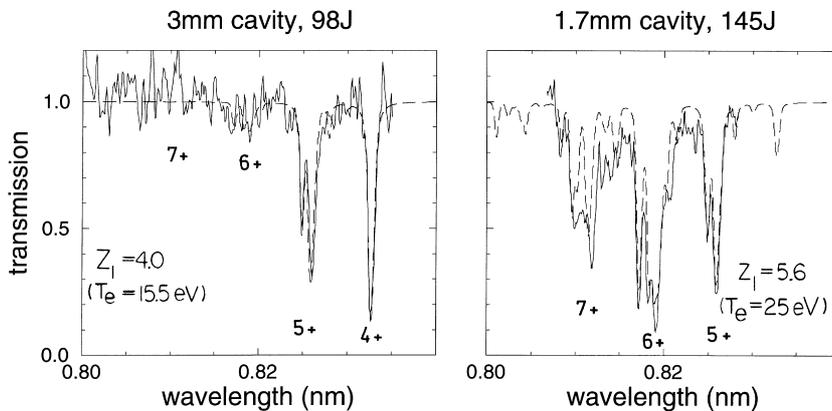
Fig. 3. Measured (solid line) and calculated (HULLAC code, dotted line) transmission spectra.  $Z_1$  is the mean ionization and  $T_e$  the electron temperature. The densities assumed are (left)  $3 \text{ mg/cm}^3$  and (right)  $10 \text{ mg/cm}^3$ .
