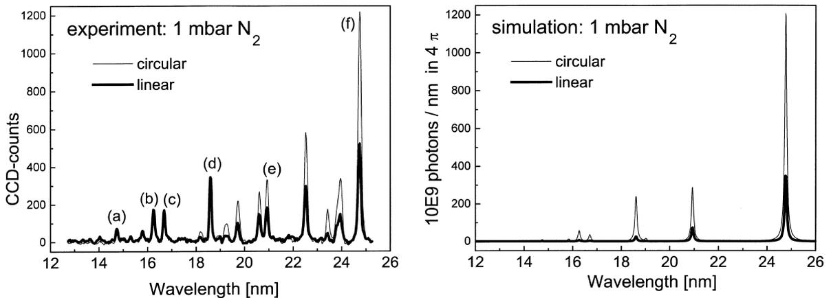
Fig. 8. (Left) Soft X-ray spectra from nitrogen.  $N^{4+}$ -lines: (a) 2s-5p, (b) 2s-4p, (c) 2p-5d, (d) 2p-4d, (e) 2s-3p, (f) 2p-3d. The other lines are due to  $N^{3+}$ . (Right) Simulated time-integrated soft X-ray spectra for  $N^{4+}$ .
