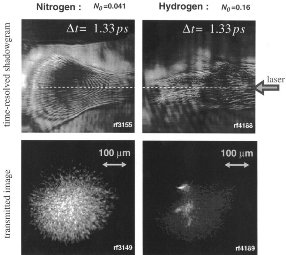
Fig. 6. Shadowgrams (upper half) taken with the  $2\omega$  probe pulse and transmitted images (lower half)  $250\ \mu\text{m}$  past focus showing the interaction of the  $0.3\ \text{TW}$  Ti:sapphire pulse with  $500\text{-}\mu\text{m}$  nitrogen and hydrogen gas jet targets.
