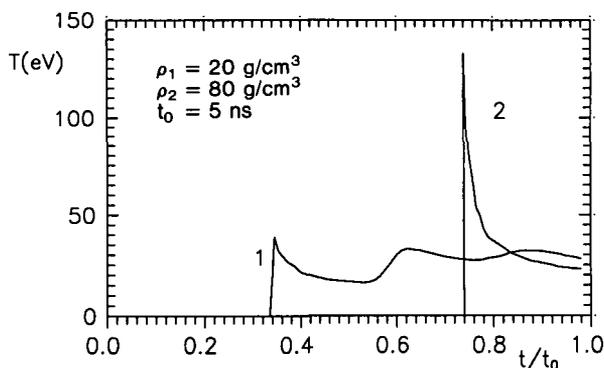
FIGURE 2. Temperature of the free boundary of the 20- $\mu\text{m}$  gold liner vs. time for two target configurations: (1),  $A_1 = 225 \mu\text{m}$ ; (2),  $A_2 = 520 \mu\text{m}$ ;  $T_1 = T_2 = 100 \mu\text{m}$ .
