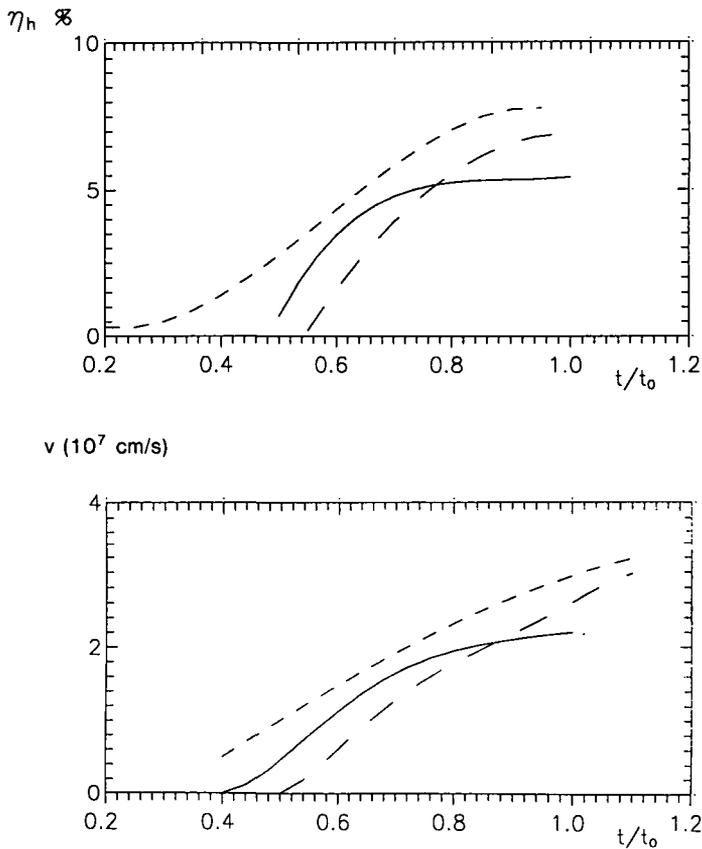
FIGURE 3. Hydrodynamic efficiency and liner velocity vs. time.
