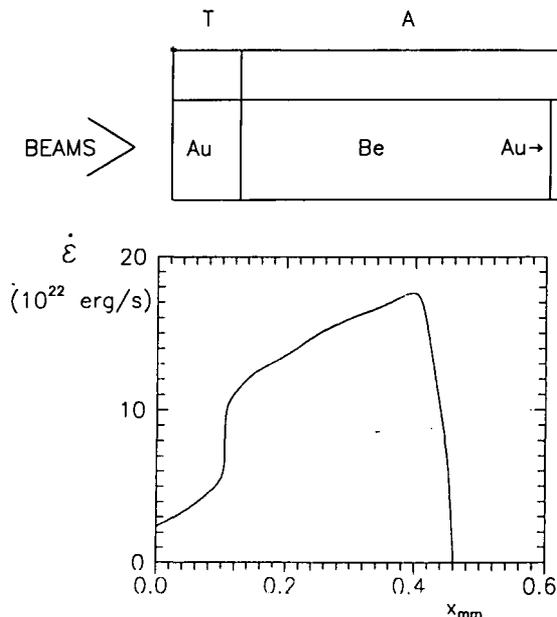
FIGURE 1. Multilayer target design and the energy deposition profile ( $T$ , tamper;  $A$ , absorber).
