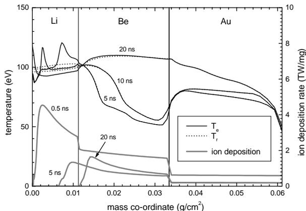
**Figure 5.** Profiles of the electron (solid curves) and radiation (dotted curves) temperatures and of the specific ion energy deposition rate (thick grey curves) at three characteristic times in case 3 of the X ray converter study.
