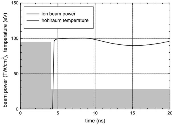
**Figure 4.** Temporal history of the radiation temperature in the middle of the hohlraum (solid curve) calculated with the step-like pulse profile (shaded area) in case 3 of the X ray converter study (Table 1).
