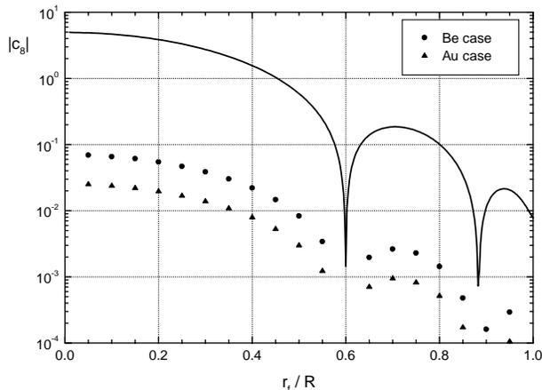
**Figure 3.** Absolute magnitude of the amplitude  $|c_8|$  (as defined by Eq. (12) and calculated with the 2-D view factor code) of the dominant  $P_8$  mode in the angular distribution of the radiation energy as a function of the ion beam focal radius  $r_f$ . Solid curve: non-uniformity of the source flux on the hohlraum wall. Circles (triangles): non-uniformity of the total energy absorbed by the fusion capsule in the case of a beryllium (gold) hohlraum wall.
