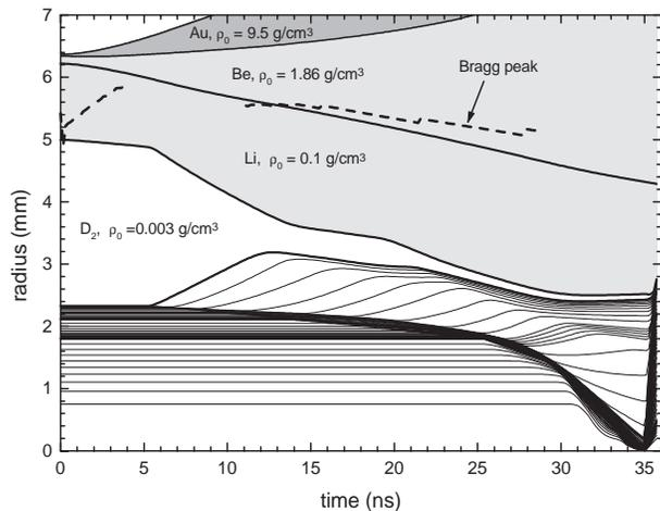
**Figure 7.** Radius–time diagram of the dynamics of the P4 target, whose initial configuration is shown in Fig. 1. The dashed line shows the position of the maximum on the ion energy deposition curve — the Bragg peak (cf. grey curves in Fig. 5).
