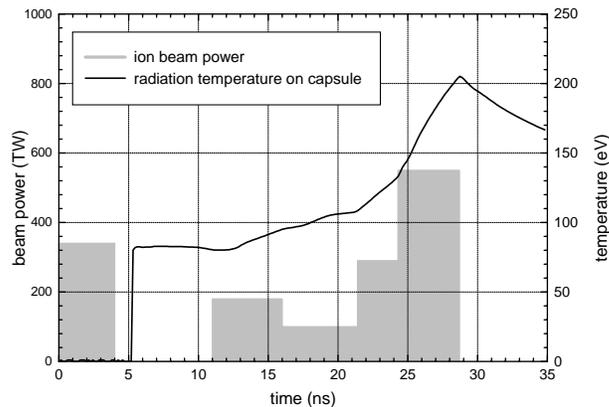
**Figure 6.** Optimized ion power pulse (shaded area) which leads to the target energy gain of  $G = 78$ . The solid curve shows the evolution of the radiation temperature at the surface of the fusion capsule.
