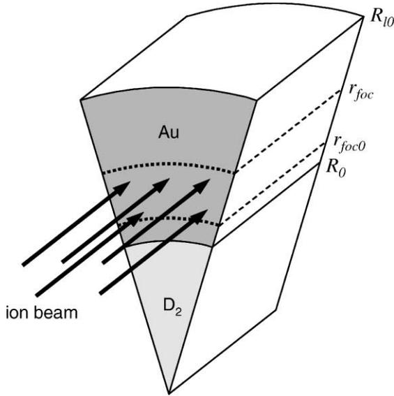
Fig. 1. Schematic view of a cylindrical target for implosion experiments with fast ion beams.
