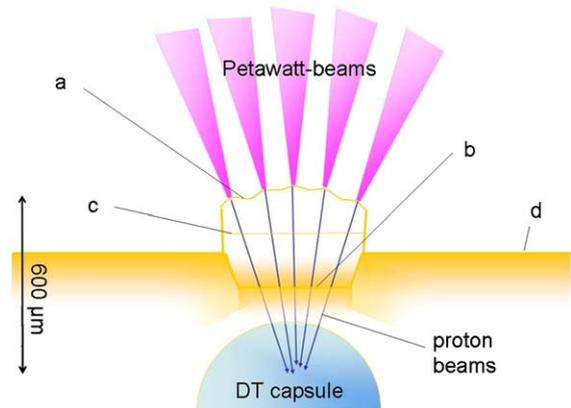
Fig. 4. Schematic for a proton fast ignition scenario with a peripheric cavity consisting of production target (a), main heat shield,  $50\ \mu\text{m}$  (b), and secondary heat shield,  $10\ \mu\text{m}$  (c) next to the main fusion cavity (d).
