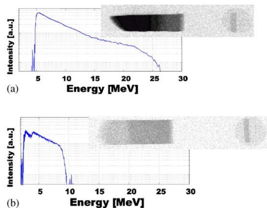
Fig. 3. Example of a proton spectrum recorded at  $I \approx 5 \times 10^{19}\ \text{W}/\text{cm}^2$  under an observation angle of  $0^\circ$  (a) and  $13^\circ$  (b). The inserted black-and-white pictures show the exposed DEF X-ray film.
