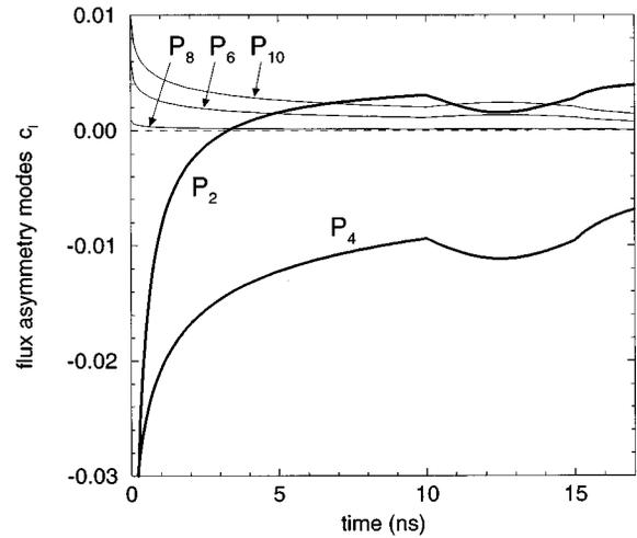
FIG. 9. Time-dependent asymmetry of capsule irradiation in a closed cylindrical hohlraum with  $R_h = 4R_c$ ,  $Z_h = R_h$ . The x-ray transfer efficiency of this hohlraum is  $\eta_h = 0.16$ .
