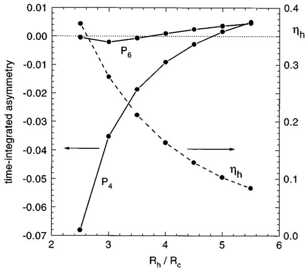
FIG. 8. Legendre components of nonuniformities in the total energy  $E_a$  absorbed by the capsule (left ordinates), and the x-ray energy transfer efficiency (right ordinates) vs the case-to-capsule radial ratio  $R_h/R_c$  in the closed cylindrical hohlraum. The source rings are placed such as to eliminate the  $P_2$  component in the time-integrated asymmetry.
