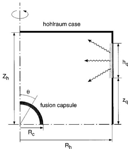
FIG. 3. Schematic one-quarter cut view of a closed cylindrical hohlraum heated by two x-ray ring sources on its sidewall. The configuration is symmetric with respect to the horizontal midplane.
