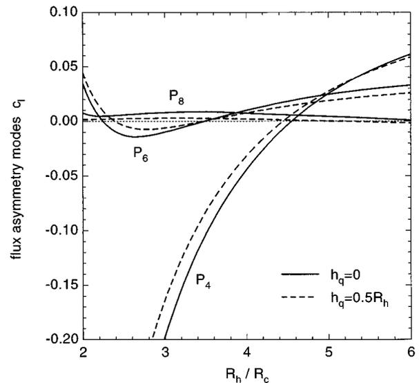
FIG. 4. Legendre components  $c_l$  of irradiation nonuniformities along the capsule surface at  $t=0$  vs the case-to-capsule radial ratio  $R_h/R_c$  in the hohlraum depicted in Fig. 3. The  $l=2$  mode is eliminated by a suitable choice of  $z_q$ . Good agreement between the dashed and solid curves demonstrates low sensitivity to the width  $h_q$  of the source rings.
